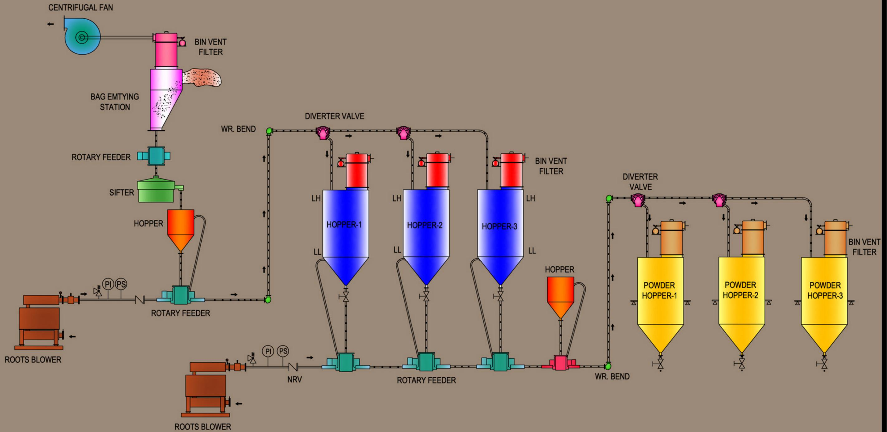
**PFD FOR CONVEYING SYSTEM FOR TOOTH PASTE INDUSTRIES**
